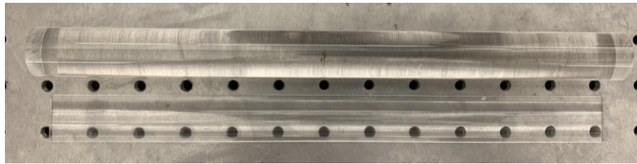
Figure 3.13 Two Kinds of Lenses. (The top is a rod lens; the bottom is a Fresnel lens)
